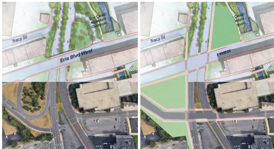
Left: NYSDOT Design for Erie Blvd and West St Interchange Right: Syracuse Urbanism Club's Flattened Intersection Design
