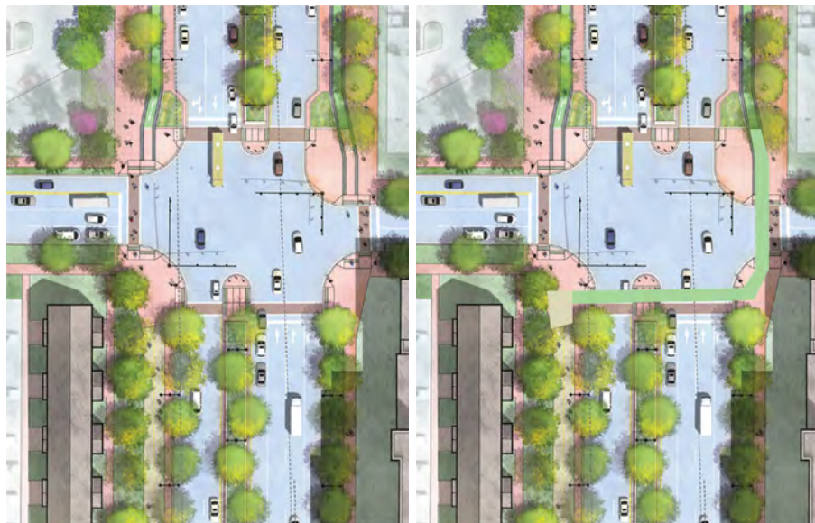
At East Adams and Almond, the transition between Almond Street's shared use path and the northbound bike lane is more clearly marked.
